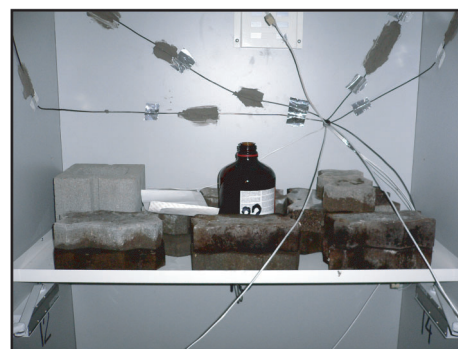
^ Sensors in a flammable cabinet
