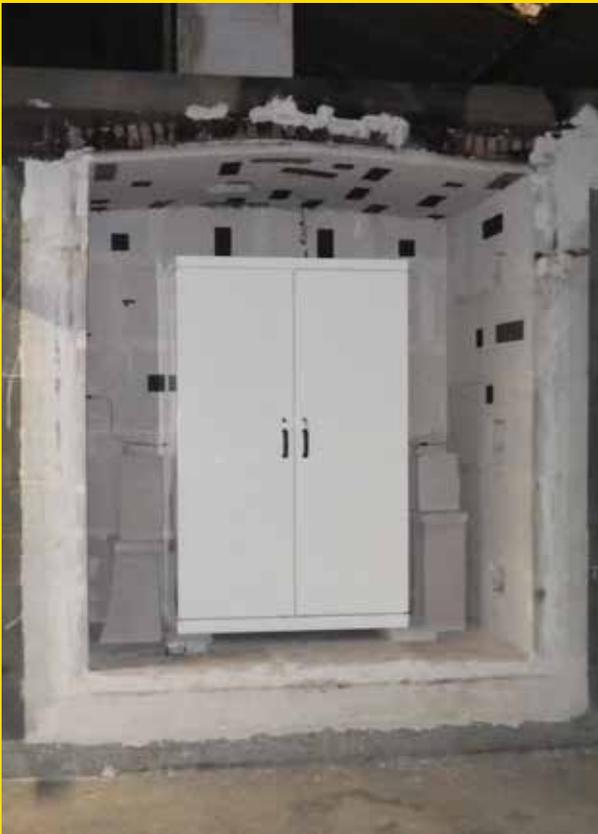
The cabinet is placed in the oven for the fire test according to EN standard. Flames will be ignited around the cabinet to simulate fire.
